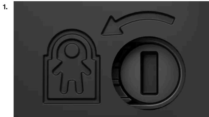
Child lock with turning direction for activation.
