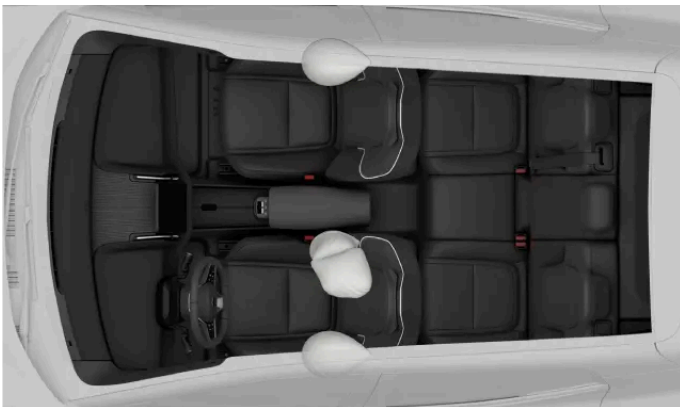
Side-on collision airbags for the front occupants.
