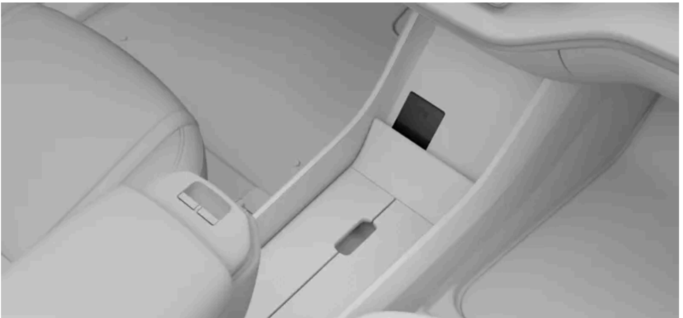
The wireless charger under the display
