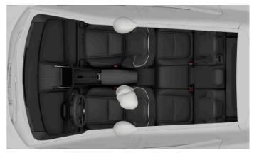
Side-on collision airbags for the front occupants.
