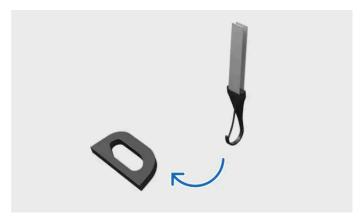
Fastening tether to lower tether attachment point
