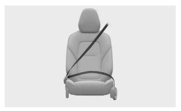
Correctly fastened and adjusted seat belt.
