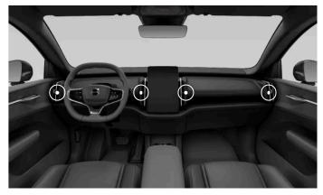
The positions of the adjustable air vents.
