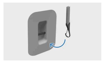
Fastening tether to top tether attachment point
