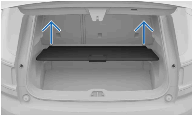
Illustrated guide to removing the cargo hatch.
