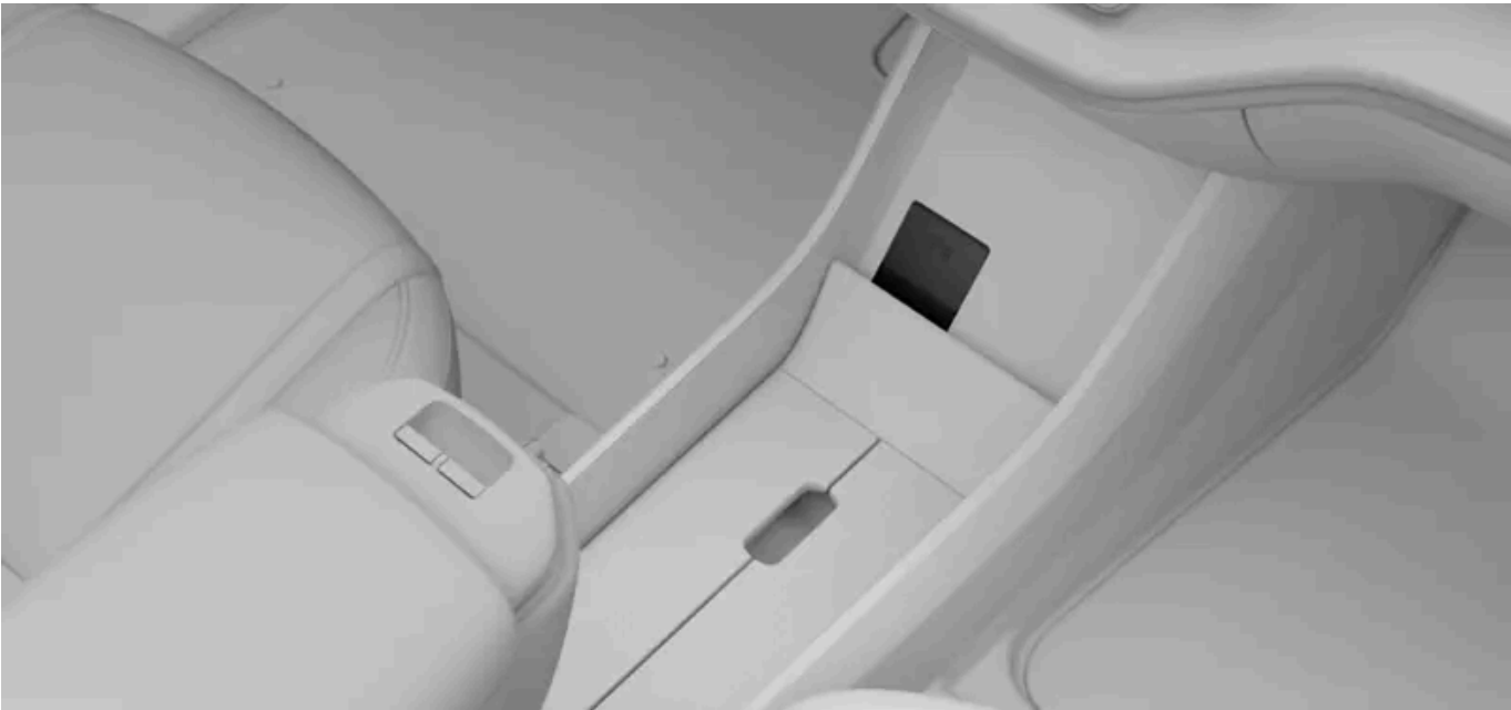
The wireless charger under the display
