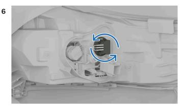
Turn the gray bulb holder counterclockwise and pull it out.
