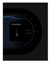
Your selected drive mode is shown above the selected gear in the instrument panel.
