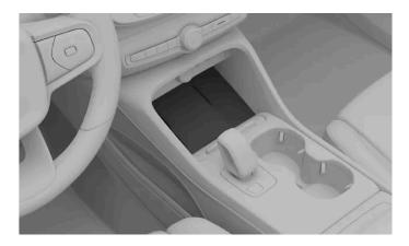
To use the wireless charger, your device should be certified to the Qi wireless charging standard. Also make sure that wireless charging is enabled on both the device [1] and on the charger itself. You can enable the charger in the center display.
