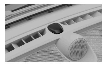
The alarm indicator is a light located in the center of the dashboard, just in front of the windshield. The indicator confirms when the alarm is enabled with a flashing red light.
