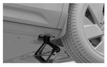
8 Raise the vehicle to an appropriate height. Do not raise it higher than necessary for the work you're doing.
