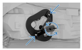
Unscrew the spring screw by turning counterclockwise. Leave the screw in the support bridge so that you can find it when you need it again.
