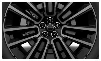
Tighten the wheel fasteners crosswise.
