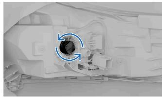
Turn the black bulb holder counterclockwise and pull it out.
