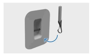
Fastening tether to top tether attachment point
