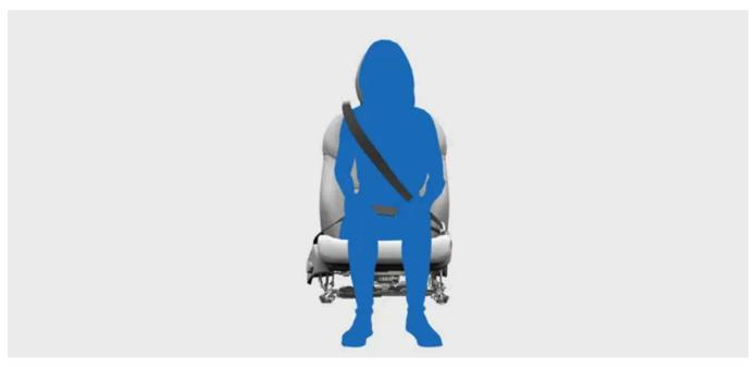
Correctly fastened and adjusted seat belt.
