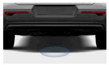
The sensor detects movement under the rear bumper. Any detected movement unlocks the trunk.
