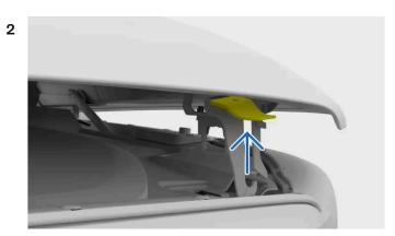
Locate the second lever on the underside of the hood and push it upward.
