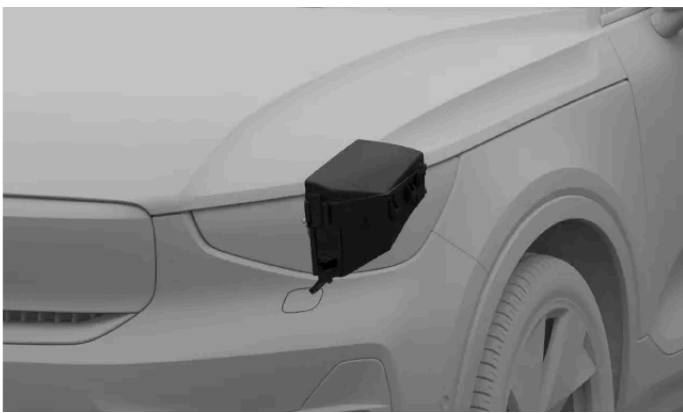
Fuse box location
