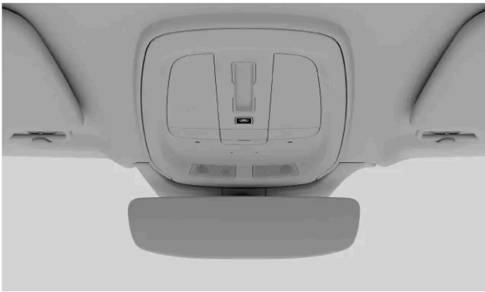
All interior lights on button in the overhead console
