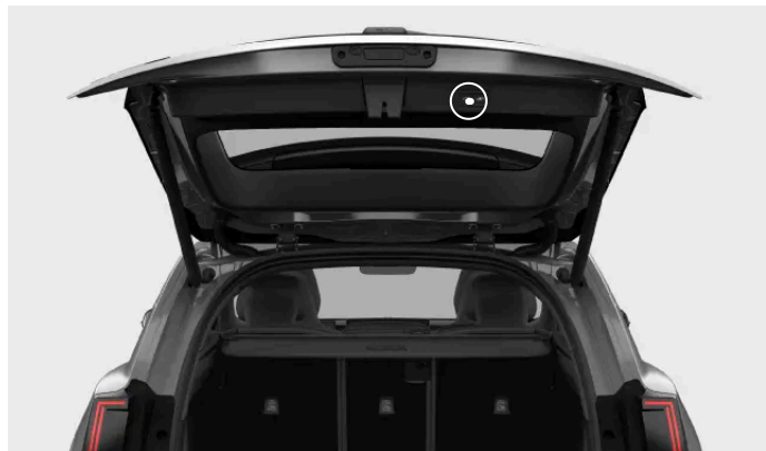
Location of the trunk closing button
