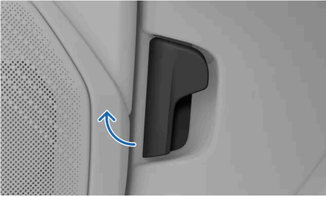
Pulling the interior release lever
