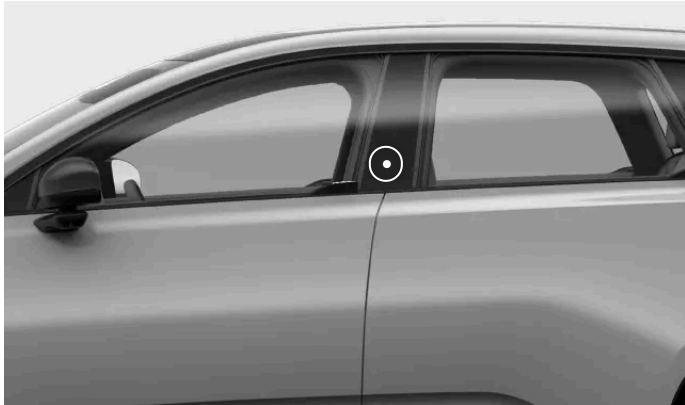
Key reading location on the driver's door pillar
