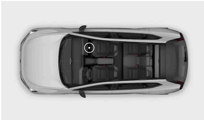
Location of VIN on the beam under the passenger seat
