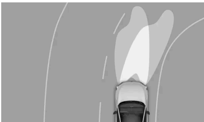
Typical function of active bending lights
