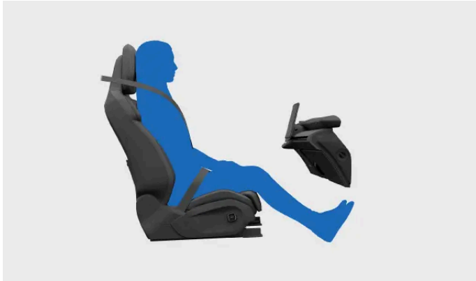
A correctly seated occupant. Do not adopt other postures when the vehicle is moving.
