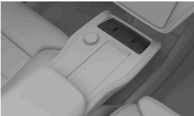
The key reader between the front seats is also the wireless charger.
