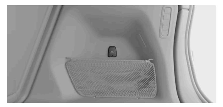
The 12 V electrical socket is on the right-hand side in the trunk.
