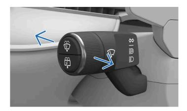
You can move the left-hand stalk forwards or backwards to switch between the different high beam options. The stalk always springs back to the neutral position.
