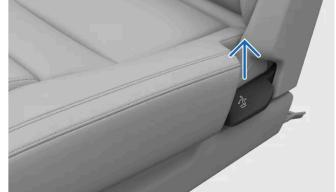
Pull and hold the handle on the side of the seat upward to unlock backrest movement.
