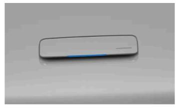
Touch point on the underside of the door handle.
