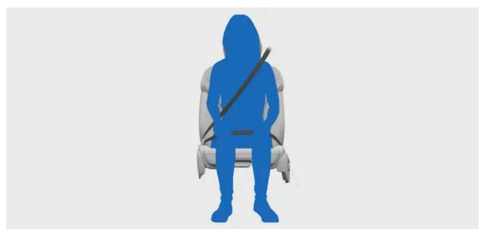
Correctly fastened and adjusted seat belt.
