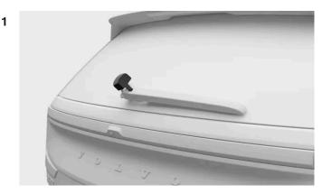
Find the plastic cover where the wiper arm attaches to the vehicle. Loosen the side of the cover closest to you first and then the side furthest away from you. Lift the plastic cover all the way. This will give you access to the hose connector.
