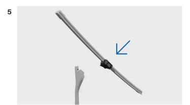
Make sure that the blade for the driver side is longer than the blade for the passenger side. Whilst keeping the wiper blade horizontal, slide the wiper blade onto the wiper arm. Ensure that the pin on the wiper arm goes into the hole on the wiper blade.
