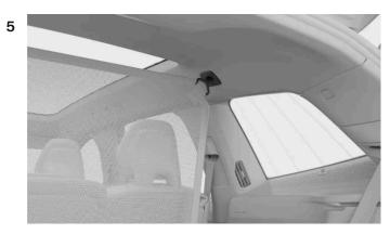
Insert each pin of the safety net into the sockets at the sides of the inner roof. Push the pins forward until they lock into place.
