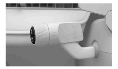
• Press and hold the button on the left-hand steering wheel stalk for the washers you want to activate. The front washers
