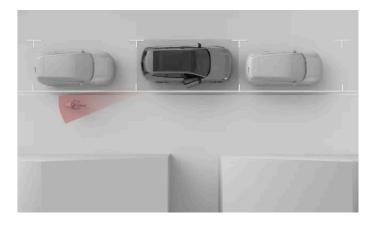
Door opening alerts are designed to warn you of passing traffic so that you don't open a door in its path. These alerts can be provided when the vehicle is stationary or moving very slowly [1].
