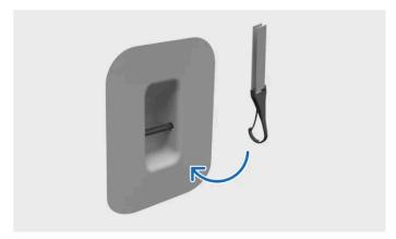
Fastening tether to top tether attachment point
