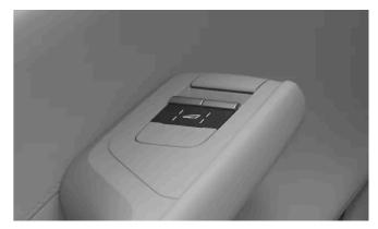
Press the window symbol at to switch between controlling the front and rear windows. The current window selection is indicated by the lights next to the symbol.
