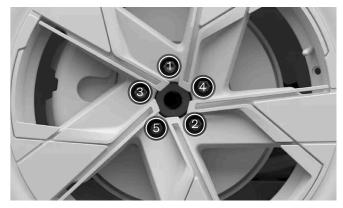
Tighten the wheel fasteners crosswise.
