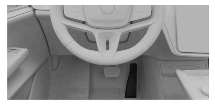
Braking behavior changes through the use of the accelerator pedal. When you press the accelerator, the vehicle accelerates normally, but releasing the pedal engages braking. The more you ease up on the pedal, the more braking action you get. By releasing the accelerator completely, you will eventually bring your vehicle to a full stop.
