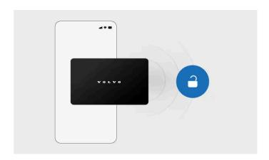
Once you've set up a digital key on your device, it works in the same way as your other keys. If your device has UWB<sup>[1]</sup> capability, your vehicle will be able to detect the digital key from a distance. If your device doesn't have UWB capability, the digital key works as a key card.
