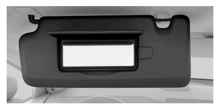
The visors can be folded down and angled to the side when necessary. With the sun visor angled to the side, you can also extend the rod holding the sun visor for better positioning.
