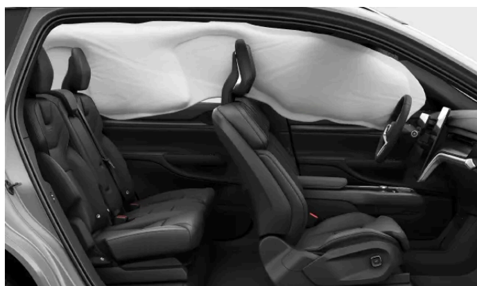
Inflatable curtain deployed on one side of the vehicle.
