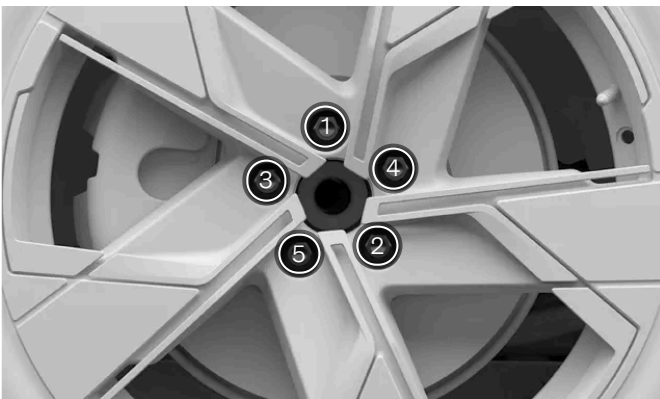
Tighten the wheel fasteners crosswise.
