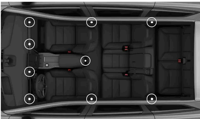
The locations of the adjustable air vents
