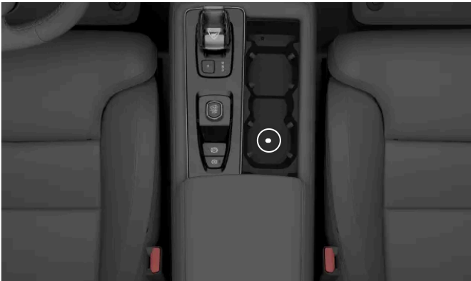
Location of the backup reader inside the center console cup holder
