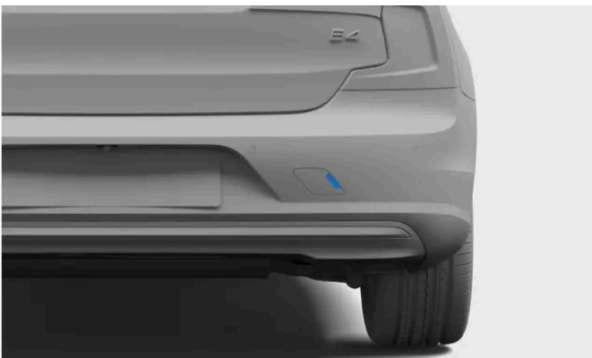
Rear towing eye fastening cover
