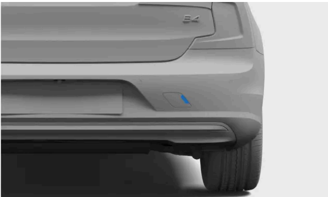
Rear towing eye fastening cover
