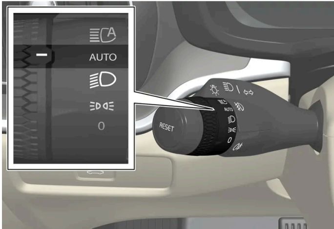
Lighting ring in AUTO position.
