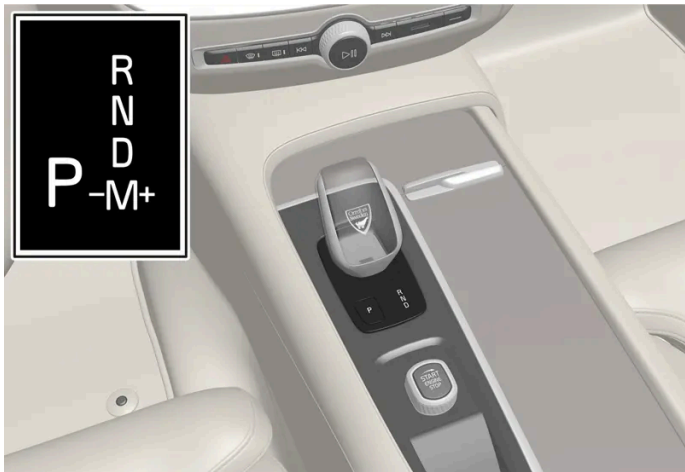
Overview of gear selector and gear shift pattern in the instrument panel.
