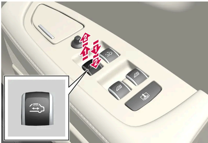
Sun curtain control.
