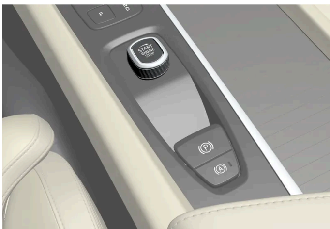
Start knob in the tunnel console.
