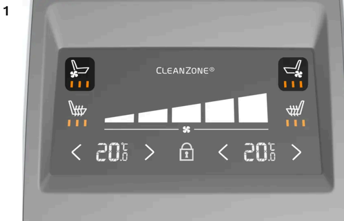
Seat ventilation controls and indicator lights on the rear side of the tunnel console.
