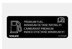
Illustration 2: Decal on the inside of the fuel filler flap on vehicles that require premium fuel [2] .
