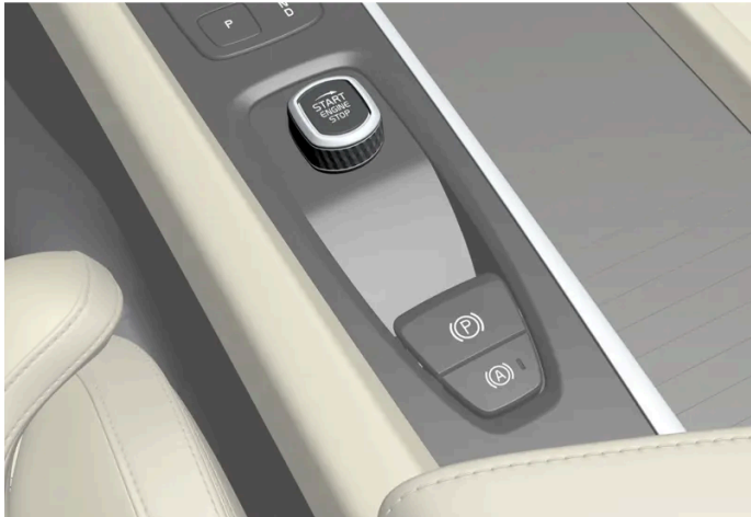
Start knob in the tunnel console.
