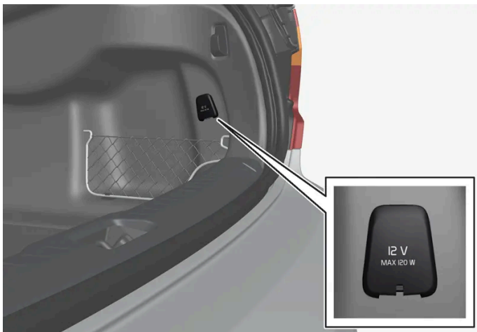
12 V outlet in trunk/cargo compartment*.
