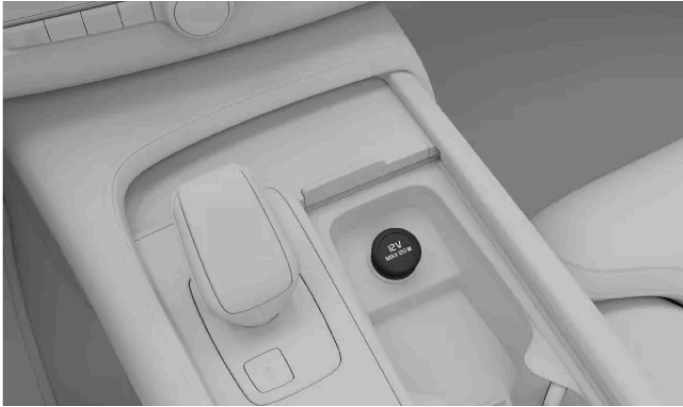
The 12 V socket in the center console
