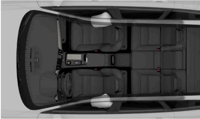
Side-collision airbags for the front occupants.
