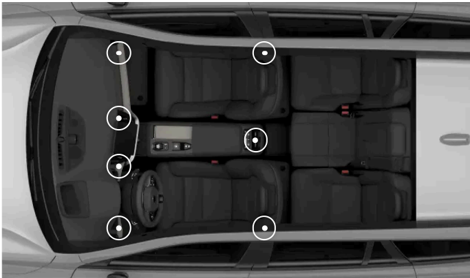
The locations of the adjustable air vents
