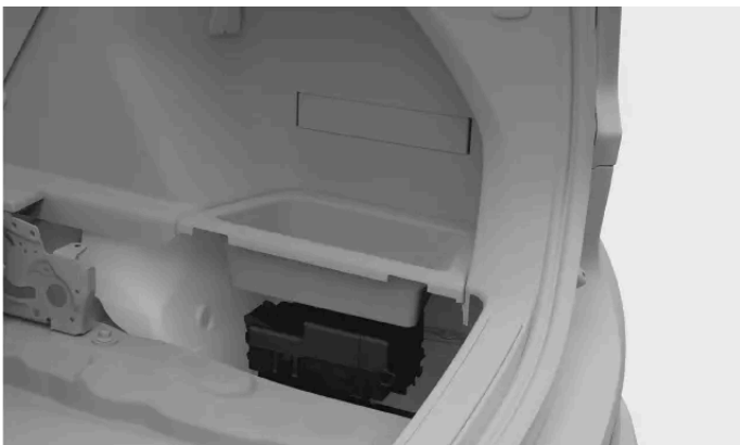
Fuse box location
