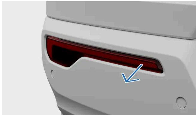
Insert a screwdriver behind the fog light's narrower short side and pry it out.
