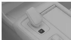
When P is selected, the transmission is mechanically blocked to avoid accidental gear shifts.
