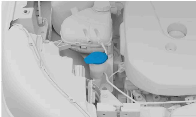
Locate the blue cap with the washer fluid symbol and open it.
