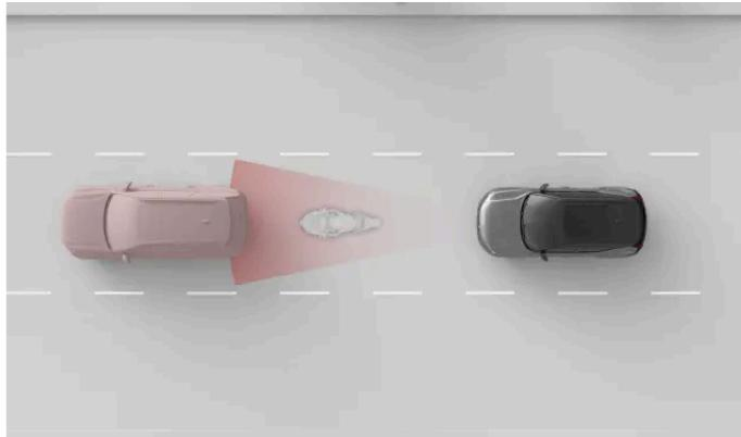
If the motorcycle and the larger vehicle are close to each other, they may appear to overlap to the detection systems, making detection of the motorcycle less accurate.
