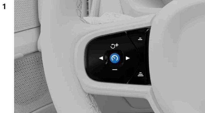
When it's safe to do so, press the Pilot Assist button
