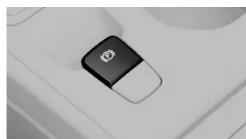
Manually engage the parking brake by pulling the parking brake switch.
