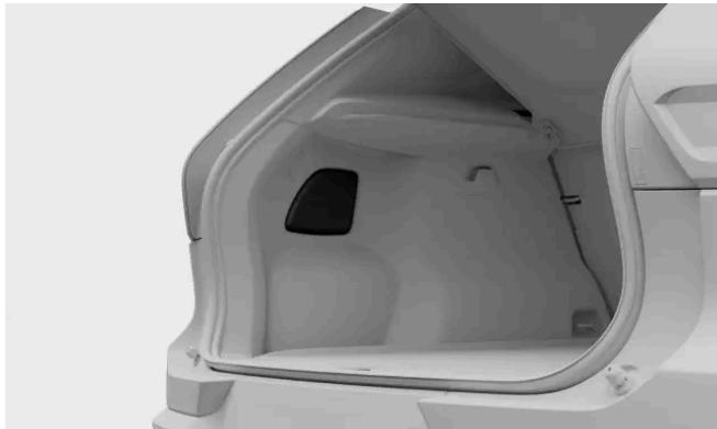
Press the top edge of the panel cover to make it pivot and remove it.
