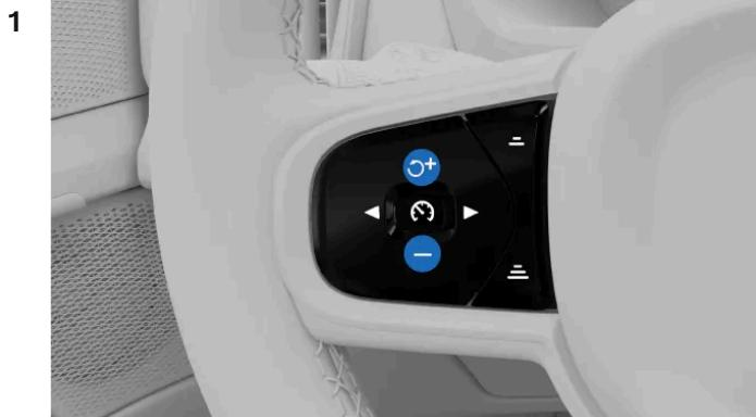
1 Adjust the target speed using the buttons on the steering wheel.
