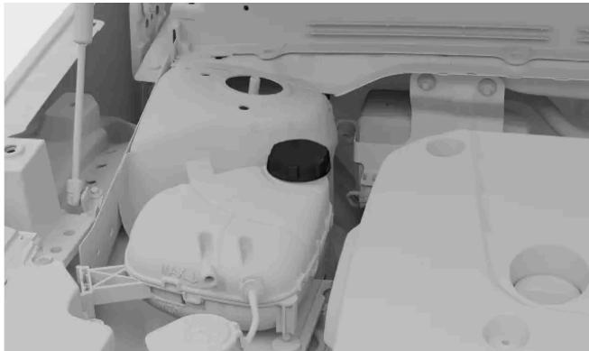
Unscrew the coolant reservoir cap.
