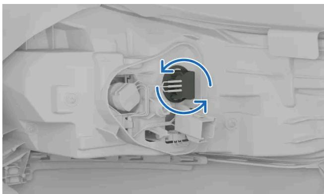
Turn the gray bulb holder counterclockwise and pull it out.
