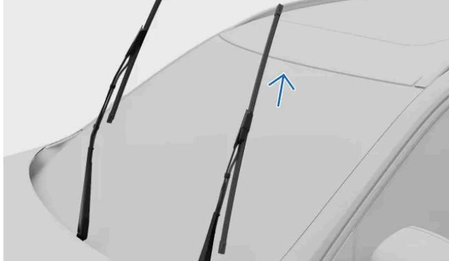
Press the button on the wiper arm and remove the wiper blade by pulling it upward.
