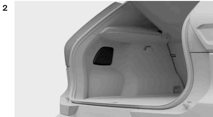
Press the top edge of the panel cover to make it pivot and remove it.
