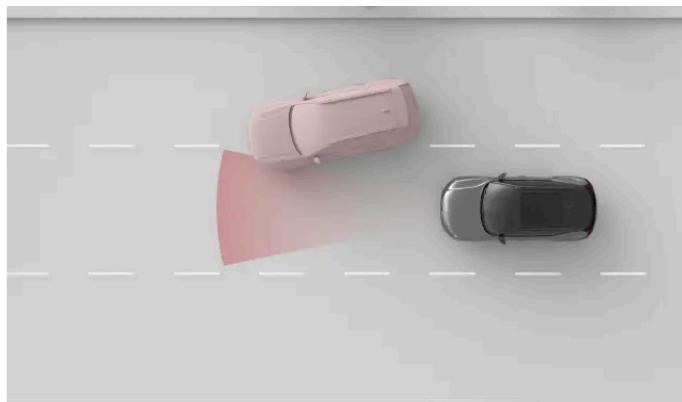
The front radar's detection zone has a limited width. If you get cut off by another vehicle, detection can occur relatively late, causing your vehicle to respond suddenly.
