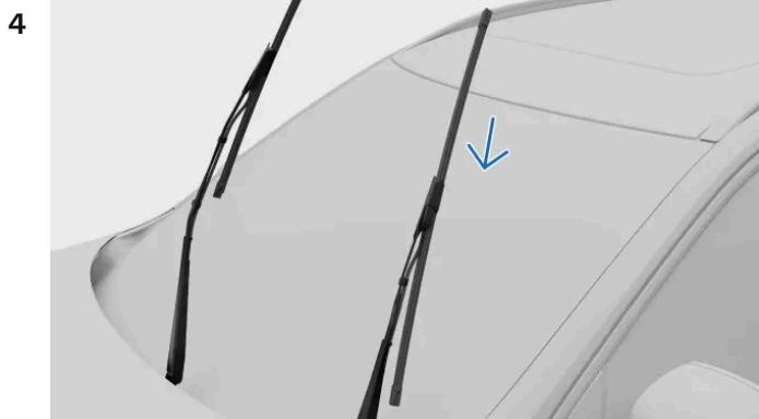
Make sure that the blade for the driver side is longer than the blade for the passenger side. Slide the wiper blade onto the wiper arm. Ensure that the pin on the wiper arm goes into the hole on the wiper blade. Push the blade into the wiper arm until you hear a click.
