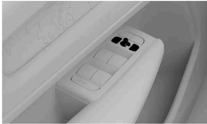
Controls for adjusting the door mirrors
