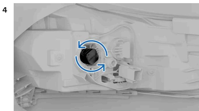
Turn the black bulb holder counterclockwise and pull it out.
