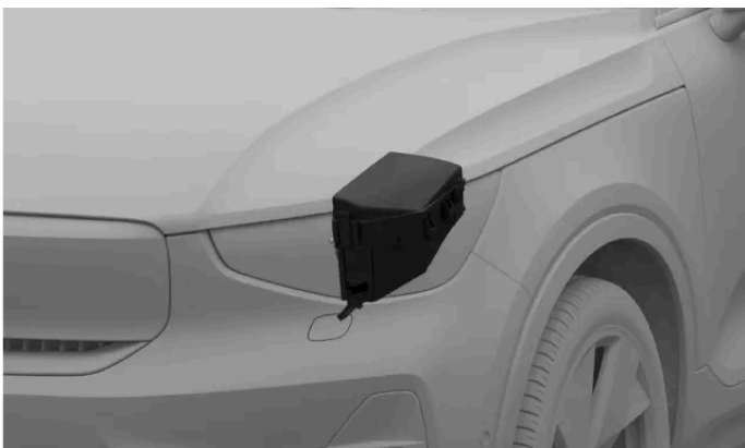
Fuse box location
