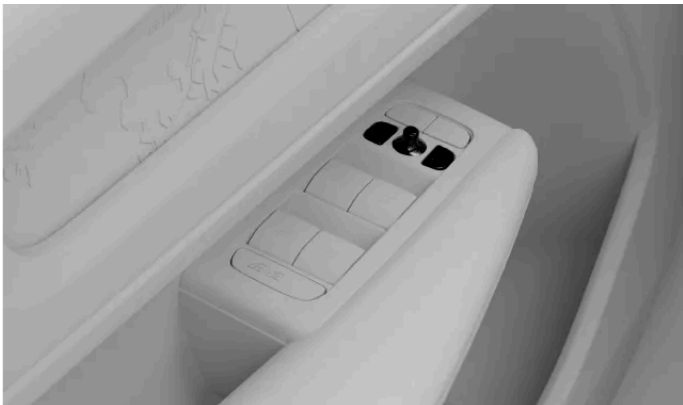
Controls for adjusting the door mirrors
