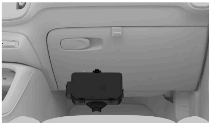
Fuse box location
