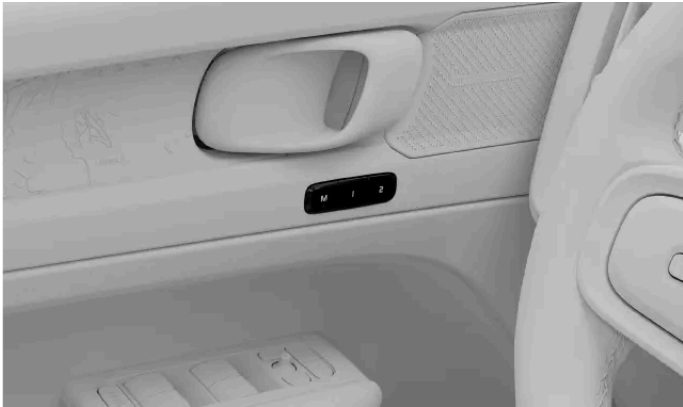
Location of the preset seat adjustment buttons
