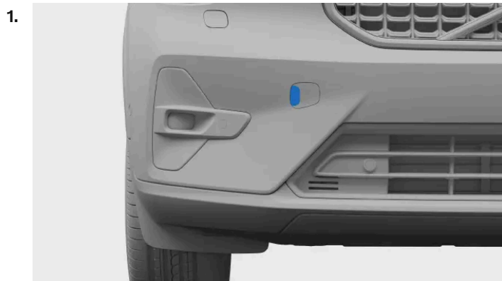
Front towing eye fastening cover
