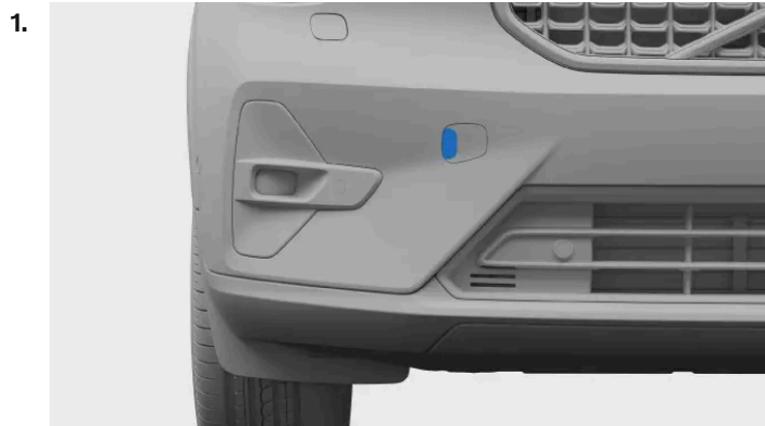
Front towing eye fastening cover
