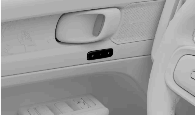
Location of the preset seat adjustment buttons
