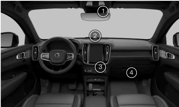
Interior climate sensors
