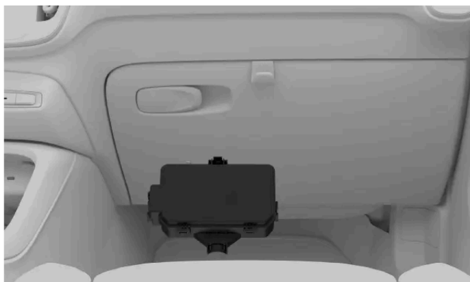
Fuse box location
