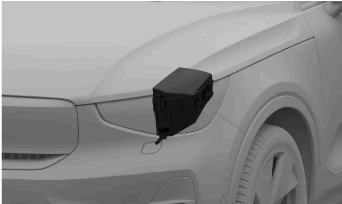
Fuse box location
