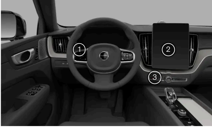
Exterior light control locations
