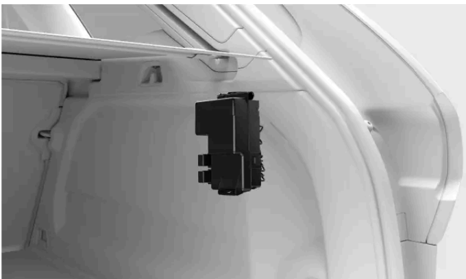
Fuse box location
