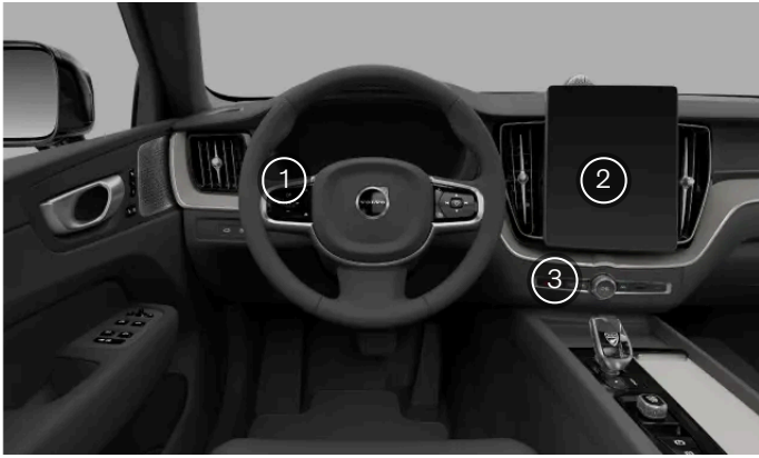
Exterior light control locations
