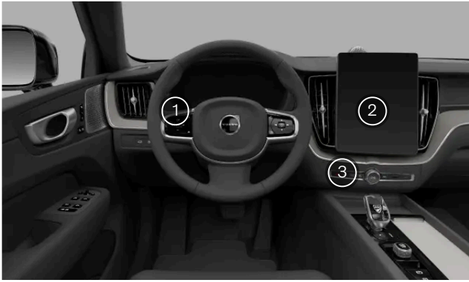
Exterior light control locations
