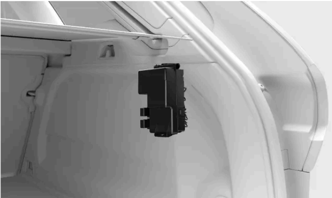
Fuse box location
