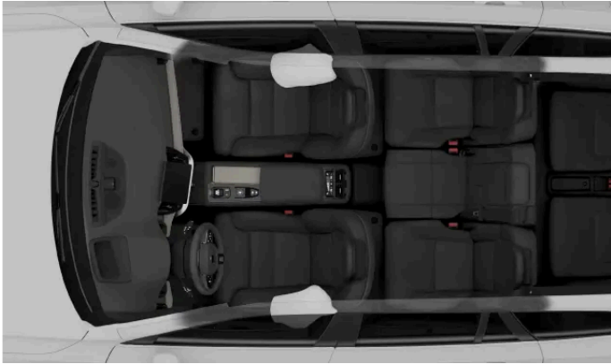
Side-collision airbags for the front occupants.
