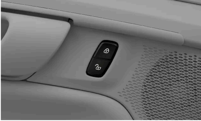
Front door button for central locking
