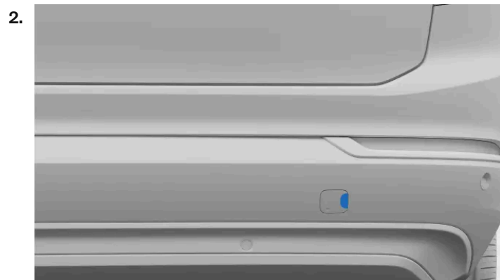
Rear towing eye fastening cover
