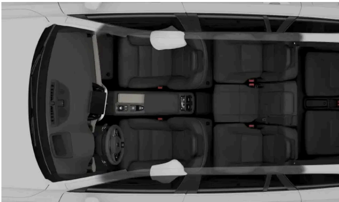
Side-collision airbags for the front occupants.
