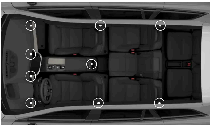
The locations of the adjustable air vents
