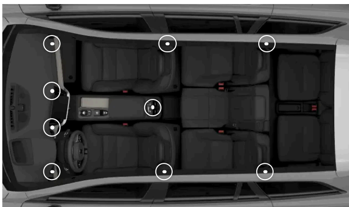
The locations of the adjustable air vents
