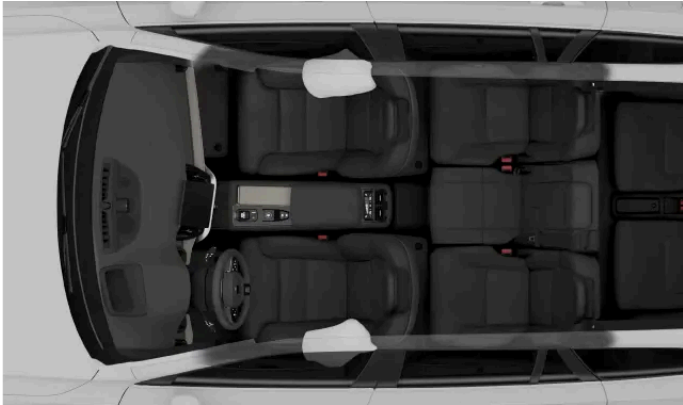
Side-collision airbags for the front occupants.
