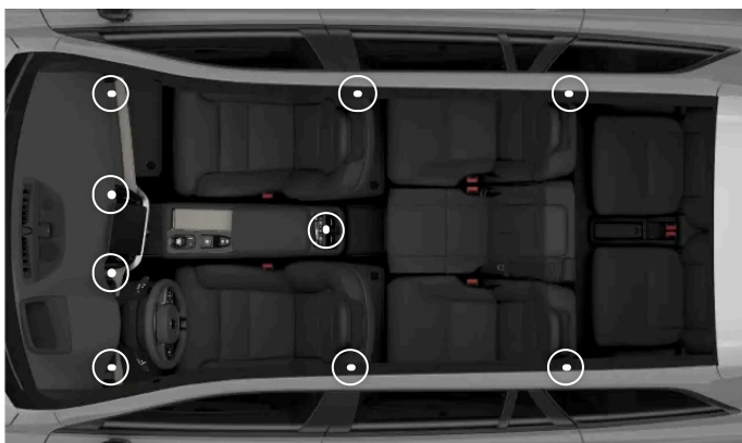
The locations of the adjustable air vents
