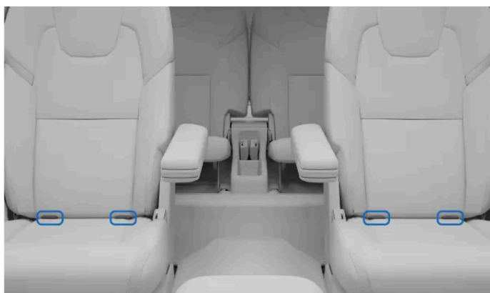
Locations of ISOFIX [1] attachment points for the second-row seats
