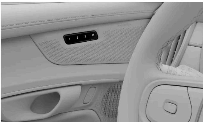
Location of the preset seat adjustment buttons
