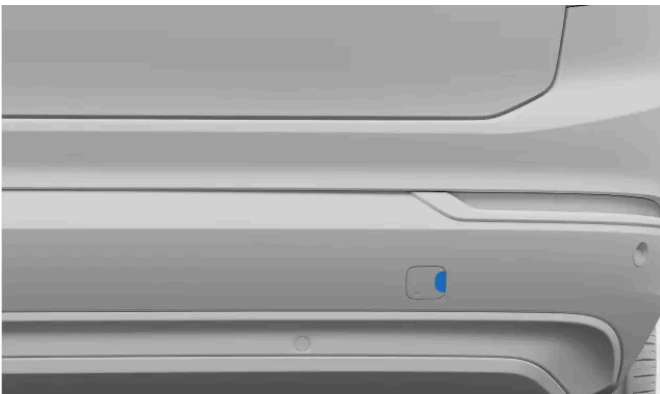
Rear towing eye fastening cover
