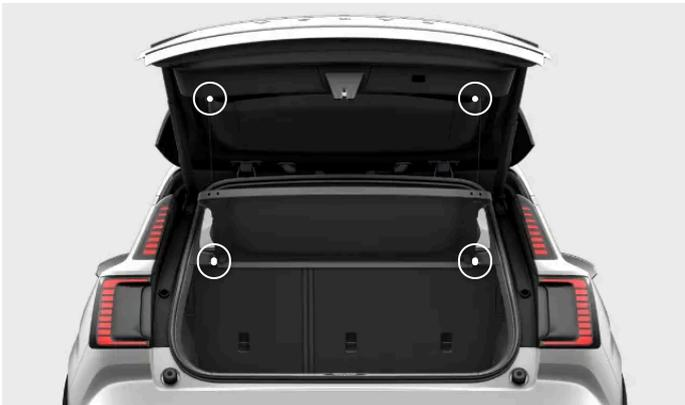
There are two attachment points on the parcel shelf itself and two on the boot hatch. When the parcel shelf is attached, cords run between attachment points on the parcel shelf and the boot hatch.
