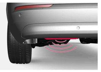
The sensor is located slightly to the left of center under the bumper.
