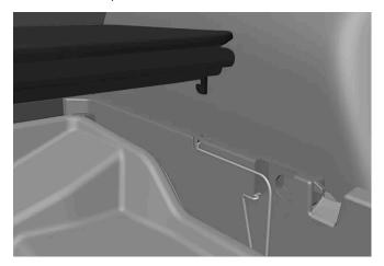
The cargo compartment floor can be carefully placed back on top of the locking clips without it locking into place.
