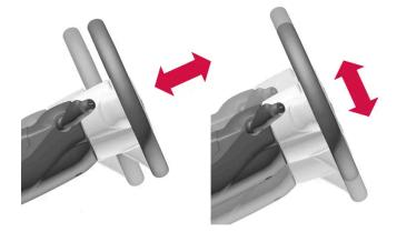
The steering wheel's reach and height can be adjusted.
