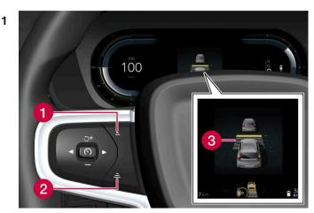
Controls for setting a time interval.
