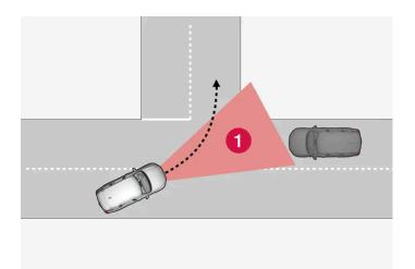
1 Sector in which the function can detect an oncoming vehicle in crossing traffic.
