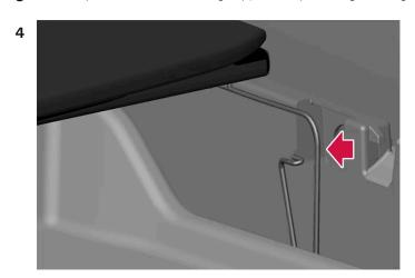
**3** Release pressure on the locking clip, but keep holding the cargo compartment floor up.
