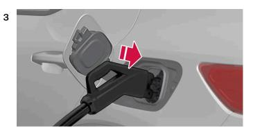
Grasp the charging cable with both hands and push the charging cable all the way into the vehicle's charging socket. Hold the charging handle up for a few seconds. The charging cable automatically locks into the charging socket after a few seconds. Make sure that the charging cable locks fully into place so that charging can start.
