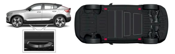
The triangles in the plastic covering indicate where the jack attachment points/lifting points (red areas) are located.
