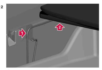
1) Press the locking clip at the location shown by the arrow until it stops. Maintain pressure on the locking clip.
