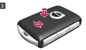
Put the front cover on in the reverse order it was removed. Press the cover down until it clicks and then push it the last few millimeters back to its original position.
