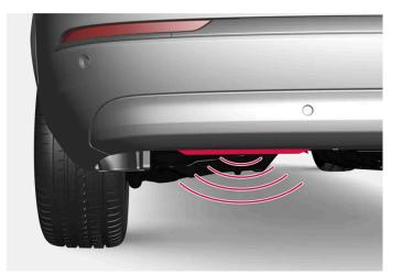
The sensor is located slightly to the left of center under the bumper.
