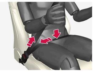
The lap section of the seat belt should be positioned low on the hips (not against the abdomen).
