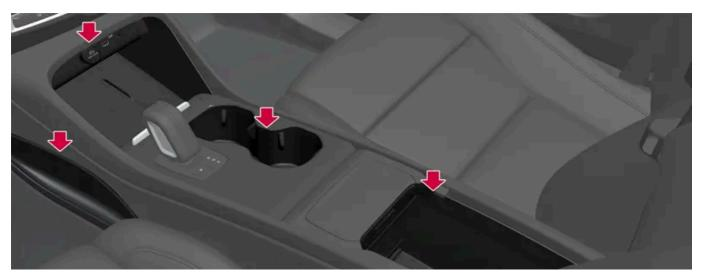
Storage compartment at leg area, electrical outlets and USB ports over the wireless phone charger\*, cup holder and storage under armrest in tunnel console.
