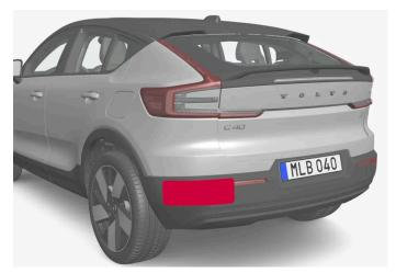
Keep the marked area clean (on both the left and right sides of the vehicle)<sup>[2]</sup>.
