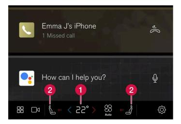
1 Temperature controls for driver and passenger side.<sup>[1]</sup>
