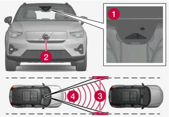
The camera and radar units monitor the distance to the vehicle ahead and detect lane markings.
