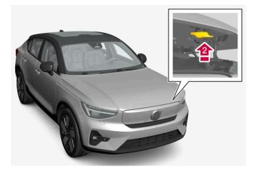
2 Move the handle under the hood upwards to release the catch and lift the hood.
