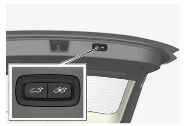
Location of button(s) on underside of tailgate.
