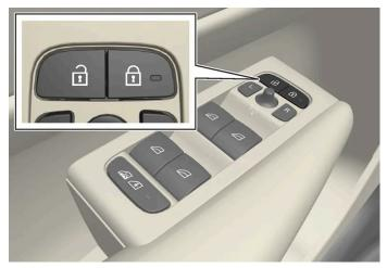
Button with indicator light for locking and unlocking in front door.
