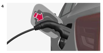
Remove the charging handle's protective cover and push the charging handle all the way into the charging socket.
