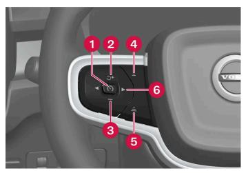
Buttons for speed-controlling functions
