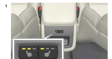
Buttons for seat heating on the rear side of the tunnel console.
