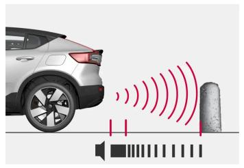
The warning signal has a continuous tone when the obstacle is less than approx. 30 cm (1 foot) from the vehicle.
