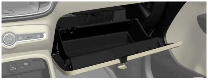
Glove compartment with fold-out hook.
