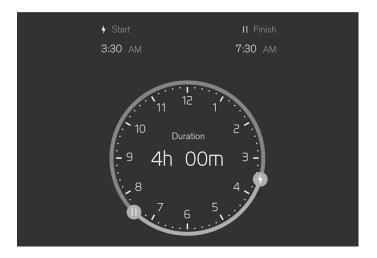
Select Charging  $\rightarrow$  Set timer in the center display and then activate the scheduled charging in Schedule charging. Drag the and | controls to set start and stop times for charging.
