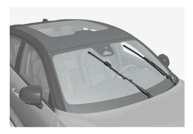
The windshield wipers must be in the service position when replacing, washing or lifting the blades (e.g. to scrape ice or snow from the windshield).
