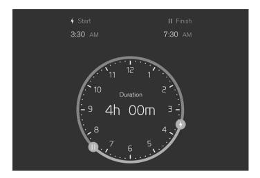
Select Charging → Set timer in the center display and then activate the scheduled charging in Schedule charging. Drag the 4 and || controls to set start and stop times for charging.
