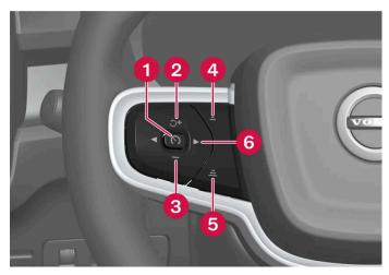
Buttons for speed-controlling functions
