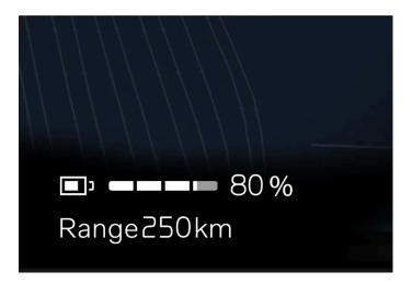
The battery gauge at the bottom of the instrument panel shows the charge level of the high-voltage battery. When the remaining range falls below 50 km (30 miles), this will be shown next to the battery gauge. Range may be affected by factors such as driving style and ambient temperature.
