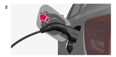
Press the lock button on the charging cable's handle. The handle will be released/unlocked. Unplug the cable from the vehicle's charging socket and close the charger door.
