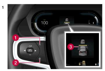
Controls for setting a time interval.
