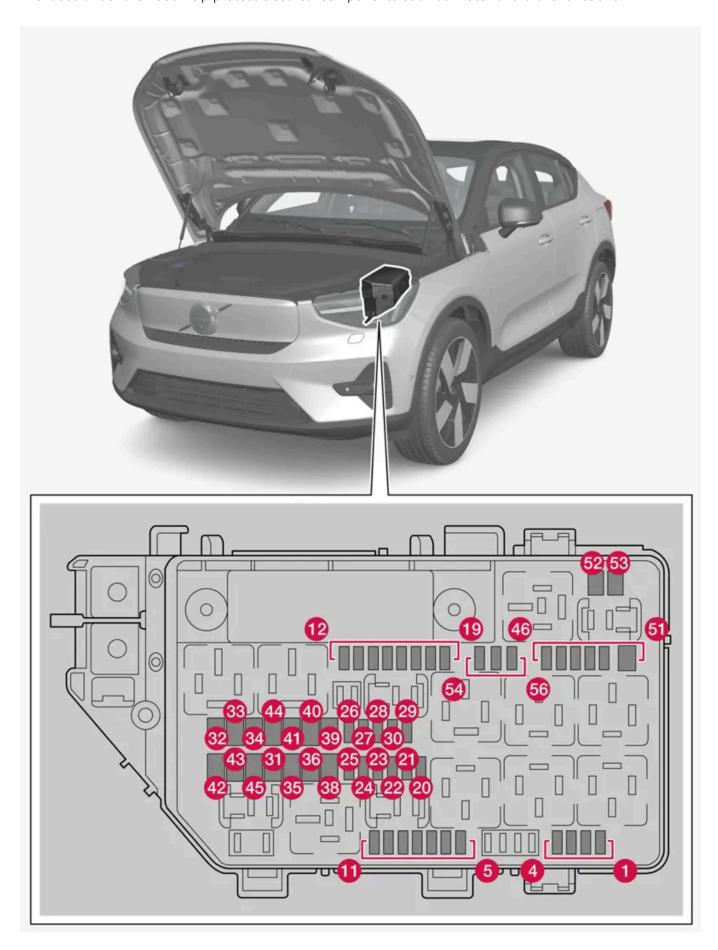
To access fuses under the hood, a number of panels around the storage compartment must be removed.
