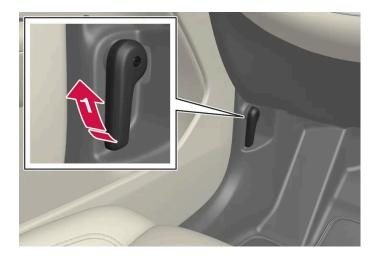
Pull the lever next to the pedals to release the hood from its fully closed position.
