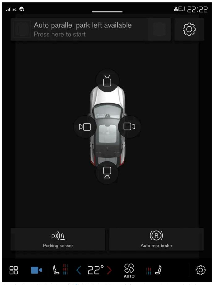
Camera view shows the Park Assist Cameras (PAC $^{[1]}$ ), which display a 360° panoramic view as well as separate views for each of the four cameras: rear, front, left and right.
