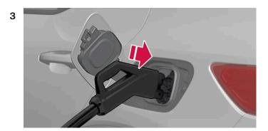
Grasp the charging cable with both hands and push the charging cable all the way into the vehicle's charging socket. Hold the charging handle up for a few seconds. The charging cable automatically locks into the charging socket after a few seconds. Make sure that the charging cable locks fully into place so that charging can start.
