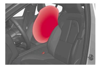
The far-side airbags are located in the front seats' inner backrest frames and help protect the driver and front-seat passenger. AIRBAG is embossed on the seat.
