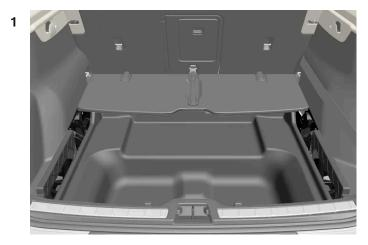
Fold the cargo compartment floor forward to position the parcel shelf with its top facing down and its rear part facing forward.
