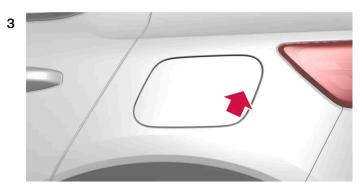
Press the rear edge of the charger door to open the charging  $socket^{[2]}$ .
