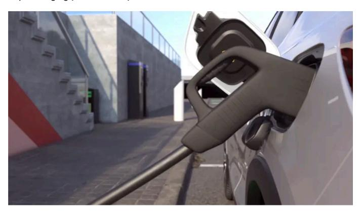
1 Remove the charging cable from the charging station's storage socket. Note that the ignition must be switched off completely before charging.
