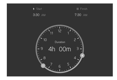
Select Charging  $\rightarrow$  Set timer in the center display and then activate the scheduled charging in Schedule charging. Drag the 4 and 11 controls to set start and stop times for charging.
