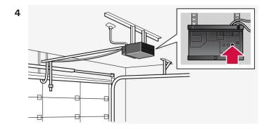
Locate the "training" button<sup>[2]</sup> on the receiver for the e.g. garage door opener. It is usually located near the antenna bracket on the receiver.
