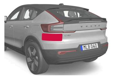
Keep the marked area clean (on both the left and right sides of the vehicle).
