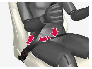
The lap section of the seat belt should be positioned low on the hips (not against the abdomen).
