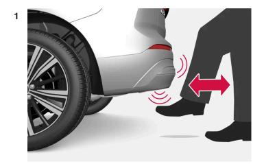
Make **one** forward kicking motion with your foot under the sensor area under the rear bumper. Then take a step back. Do not touch the bumper.
