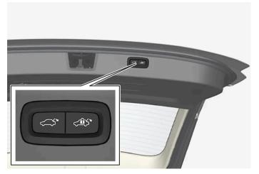
Location of button(s) on underside of tailgate.
