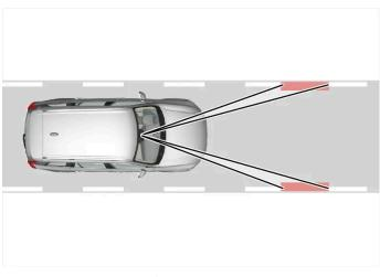
Driver Alert detects the vehicle's position in the traffic lane.
