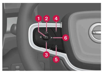
Buttons for speed-controlling functions
