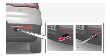
Front: Remove the cover by pressing the cover. The cover turns along its center line and can then be removed.
