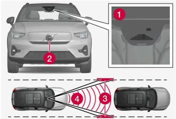
The camera and radar units monitor the distance to the vehicle ahead and detect lane markings.
