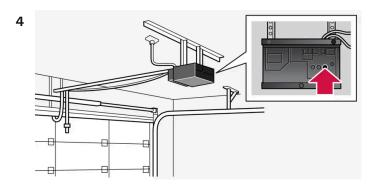
Locate the "training" button [2] on the receiver for the e.g. garage door opener. It is usually located near the antenna bracket on the receiver.
