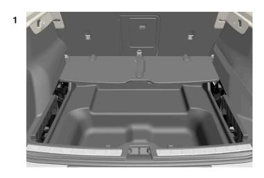
Push the folding cargo compartment floor forward so that it folds together.
