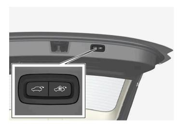
Location of button(s) on underside of tailgate.
