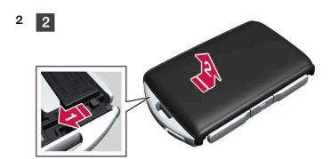
Move the catch behind the front cover to the side and slide the rear cover away from the key ring bracket.
