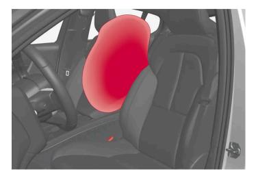
The far-side airbags are located in the front seats' inner backrest frames and help protect the driver and front-seat passenger. AIRBAG is embossed on the seat.
