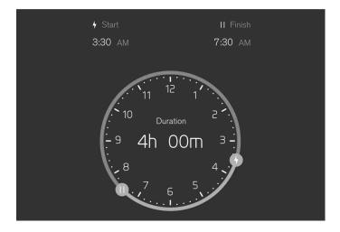
Select Charging → Set timer in the center display and then activate the scheduled charging in Schedule charging. Drag the 4 and 11 controls to set start and stop times for charging.
