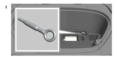
Take out the towing eyelet, which is stored in a foam block under the hood.
