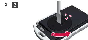
Turn the battery cover counterclockwise to the OPEN position. Use a screwdriver, coin or similar.
