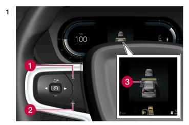
Controls for setting a time interval.
