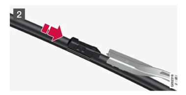
Make sure that the windshield wipers are in service position and raise the wiper blades. Service position is activated and deactivated via the center display when the vehicle is stationary and the windshield wipers are not on.
