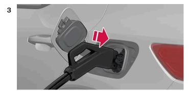
Grasp the charging cable with both hands and push the charging cable all the way into the vehicle's charging socket. Hold the charging handle up for a few seconds. The charging cable automatically locks into the charging socket after a few seconds. Make sure that the charging cable locks fully into place so that charging can start.
