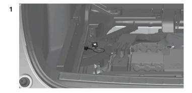
Open the vehicle's cargo compartment and lift up the rear edge of the cargo compartment floor. Lift off the recessed floor panel.
