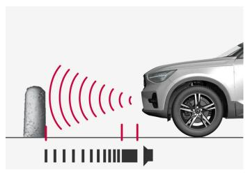
The warning signal has a continuous audible tone when the obstacle is less than approx. 30 cm (1 foot) from the vehicle.
