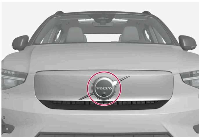
Location of the front radar sensor
