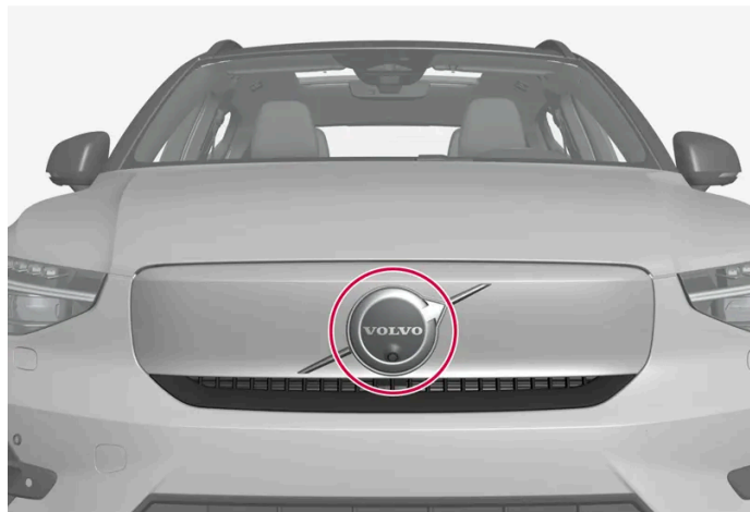
Location of the front radar sensor
