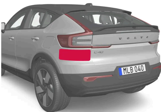
Location of rear radar sensors
