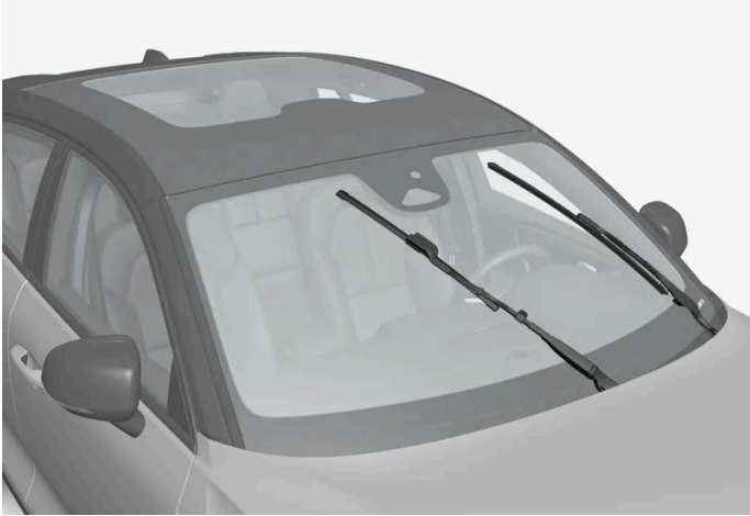
Windshield wipers in the service position.
