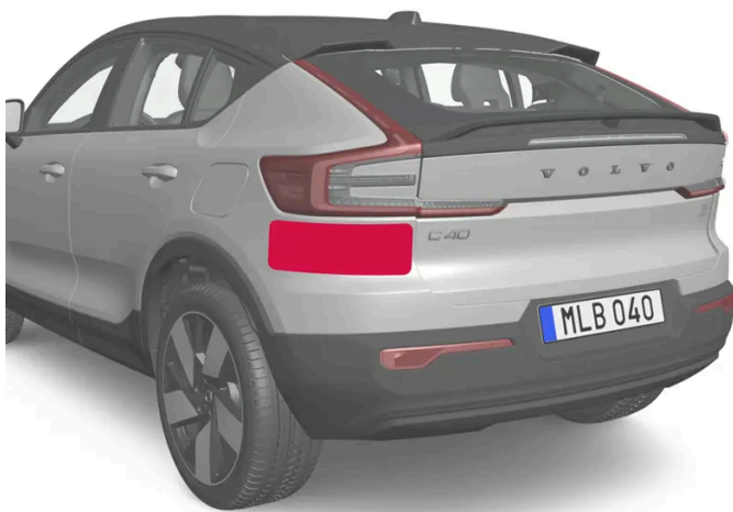
Location of rear radar sensors
