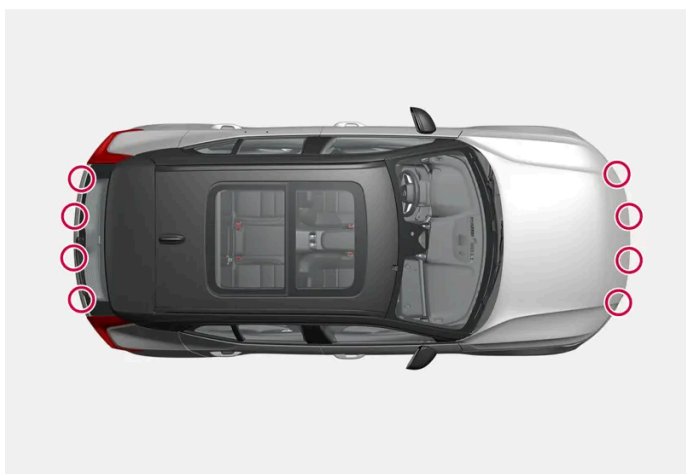
Location of the parking sensors around the vehicle
