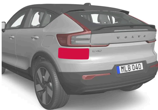
Location of rear radar sensors
