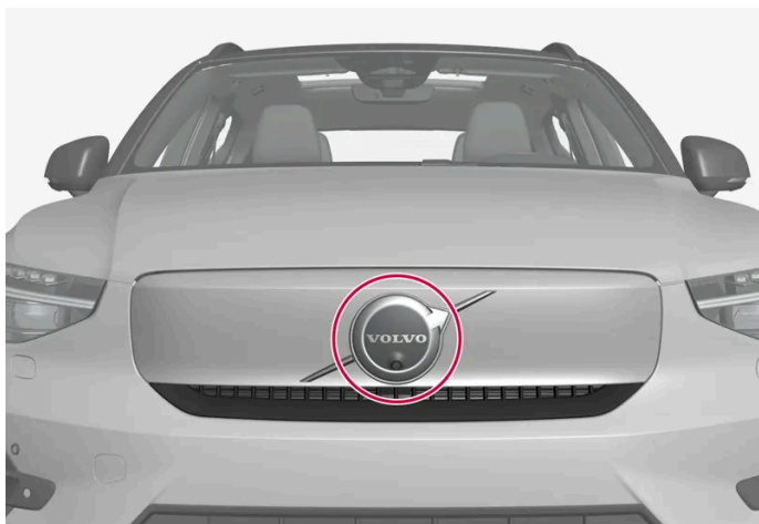
Location of the front radar sensor
