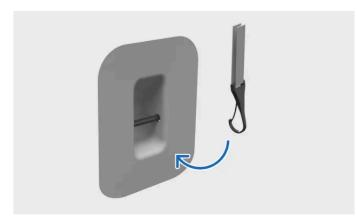
Fastening tether to top tether attachment point
