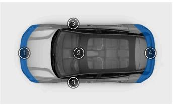
1) The front of the vehicle houses several detection components. There is a radar in center, just below the license plate, as well as additional radar units in each corner. There is also a camera in the center and several parking sensors along the lower edge.
