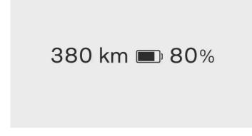
The battery meter is shown in the driver information area at all times. The battery icon's color changes depending on the level of charge remaining on the battery.
