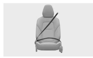
Correctly fastened and adjusted seat belt.
