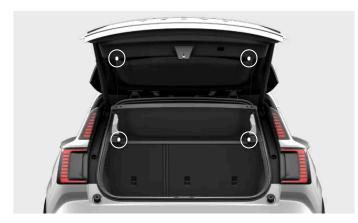
There are two attachment points on the parcel shelf itself and two on the boot hatch. When the parcel shelf is attached, cords run between attachment points on the parcel shelf and the boot hatch.
