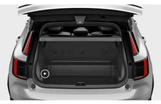
**3** Remove the cap by prying it off with a screwdriver or a similar tool.
