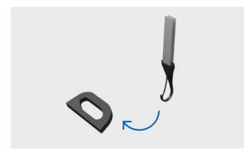
Fastening tether to lower tether attachment point
