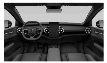
The positions of the adjustable air vents.
