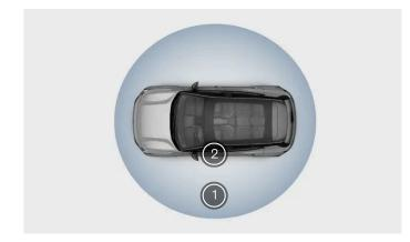
1) Distance-capable keys can lock or unlock the vehicle from a distance.
