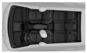
Side-on collision airbags for the front occupants.
