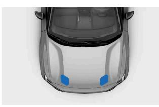
Press down with both hands on the front edge of the hood. Make sure the hood fits into the latches at the same time. Keep the front edge flat as it closes.
