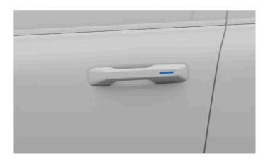
When using your digital key, if the proximity lock function is turned off in settings, you need to manually lock the vehicle. You do this by placing your thumb at a specific point on the driver door handle.
