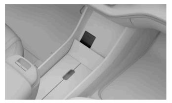
The location of the key card reader used to start the vehicle with a key card or a discharged distance-capable key.
