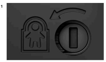
Child lock with turning direction for activation. Insert a tool into the switch hole.
