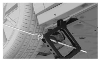
7 Raise the vehicle to an appropriate height. Do not raise it higher than necessary for the work you're doing.
