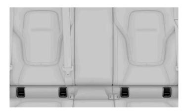
The ISOFIX<sup>[1]</sup> attachment points for the rear seats are located behind a flap in the lower part of the backrest on the outer rear seats. The flap needs to be unfolded to access the anchor points behind it.
