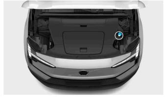
Locate the blue cap with the washer fluid symbol and open it.
