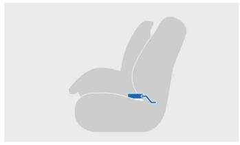
Child restraint installed using ISOFIX<sup>[1]</sup>
