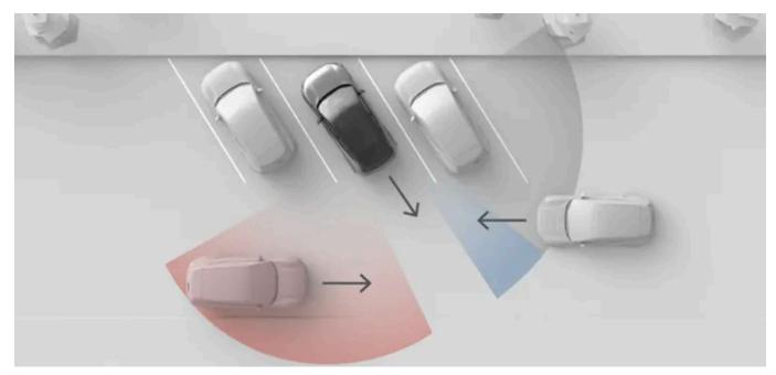
The situation shown in this image illustrates how surrounding objects, such as parked vehicles, can limit the radar's view. In a situation without obstacles, the effective detection zones are the same on both sides.
