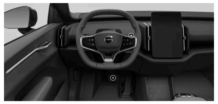
Your main interaction points for starting your vehicle are the brake pedal and the gear stalk.
