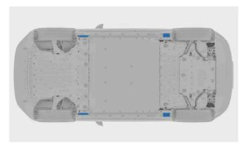
There are two jacking points on each side of the vehicle.
