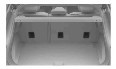
The top tether attachment points for the rear seats are located on the back of the rear seats.
