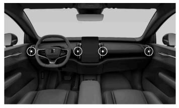
The positions of the adjustable air vents.
