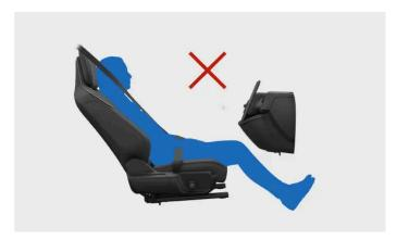
Do not fold the backrest to a lying position. The seat belt must remain tensioned against the shoulder.
