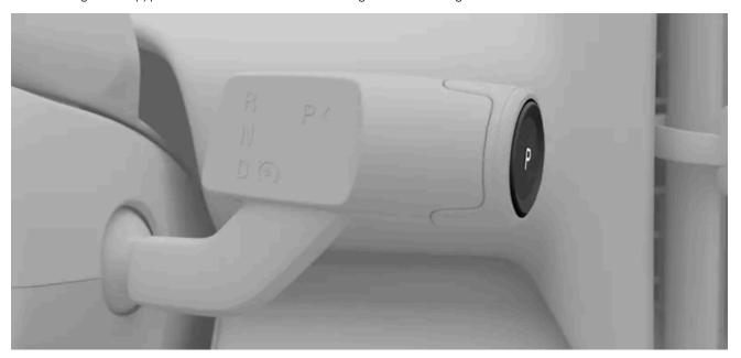
> The vehicle transitions to a parked state, which includes engaging the parking brake. The new state is indicated in the driver information area.
