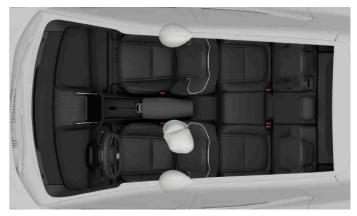
Side-on collision airbags for the front occupants.
