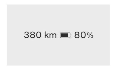
Your range is primarily related to your vehicle's battery level and your driving practices, but external conditions can also be a factor. The battery level and expected range are displayed in the driver information area. The expected range tells you how far you can drive with the current battery level. It is calculated based on your driving pattern, both current and historical, and on real-time driving conditions.
