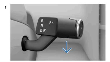
When appropriate, pull the right-hand steering wheel stalk all the way down.
