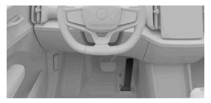
Braking behavior changes through the use of the accelerator pedal. When you press the accelerator, the vehicle accelerates normally, but releasing the pedal engages braking. The more you ease up on the pedal, the more braking action you get.
