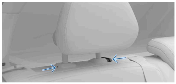
Buttons used to remove headrest.
