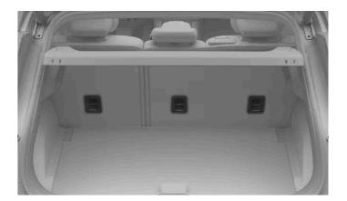
The top tether attachment points for the rear seats are located on the back of the rear seats.
