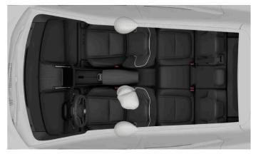
Side-on collision airbags for the front occupants.
