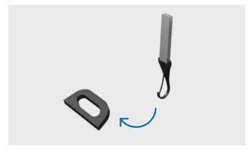
Fastening tether to lower tether attachment point
