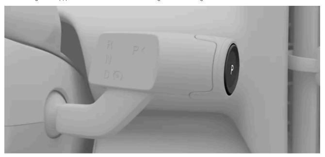
> The vehicle transitions to a parked state, which includes engaging the parking brake. The new state is indicated in the driver information area.
