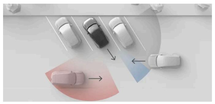
The situation shown in this image illustrates how surrounding objects, such as parked vehicles, can limit the radar's view. In a situation without obstacles, the effective detection zones are the same on both sides.
