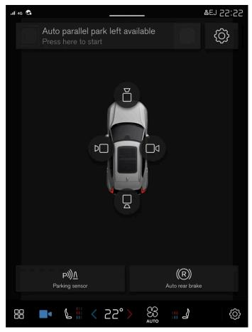
Camera view shows the Park Assist Cameras (PAC<sup>[1]</sup>), which display a 360° panoramic view as well as separate views for each of the four cameras: rear, front, left and right.
