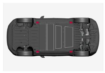
The vehicle's lifting points for lifting with a jack.
