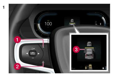
Controls for setting a time interval.
