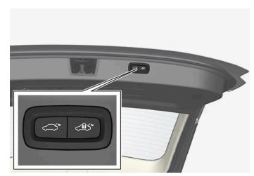
Location of button(s) on underside of tailgate.
