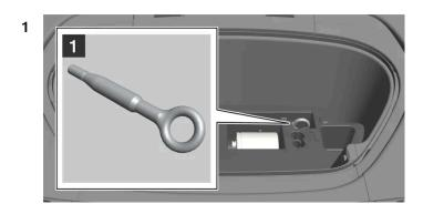
Take out the towing eyelet, which is stored in a foam block under the hood.
