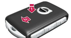
Turn the key and put the front cover back on in the same way as the back cover.
