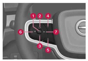
Buttons for speed-controlling functions
