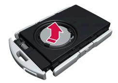
The battery's positive side (+) faces upward. Remove the battery by pressing its edge and then lifting it out.
