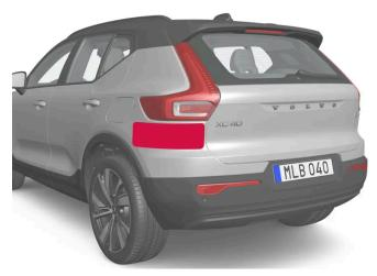
Keep the marked area clean (on both the left and right sides of the vehicle).
