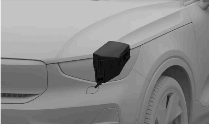
Fuse box location
