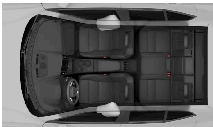
Side-collision airbags for the front occupants.
